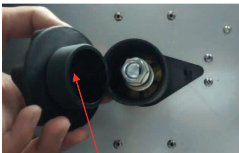
(1) Remove the spool retaining nut.
